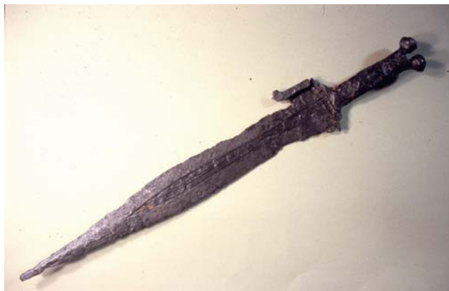
Fig. 8 Celtiberian sword from Uxama, after electrochemical cleaning. Some active pitting corrosion can be seen (photograph taken in 1998)
