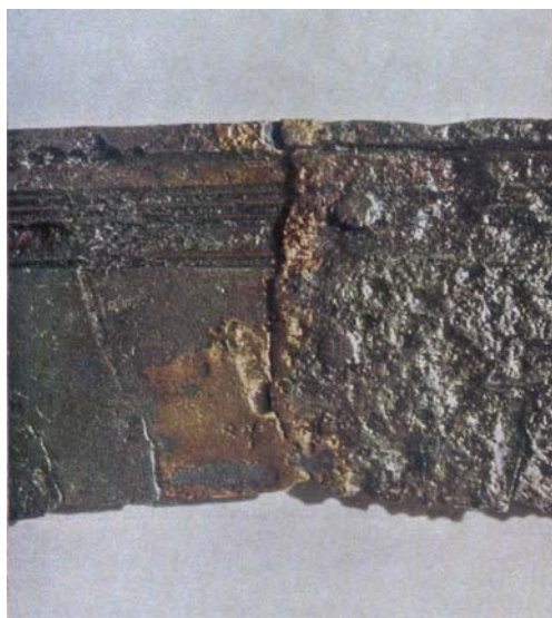
Fig. 5 Detail of the central area of the falcate sword from Almedinilla. On the right , the typical outline produced by electrolytic cleaning can be appreciated [14]
